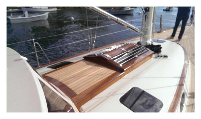
Custom teak and stainless-steel opening skylight and flush opening deck hatches.
