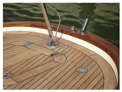
Aft deck – custom flag socket for dinghy towing, stainless steel hydraulic backstay, and flush plate for fresh water hot/cold deck shower FRIENDSHIP YACHT COMPANY
