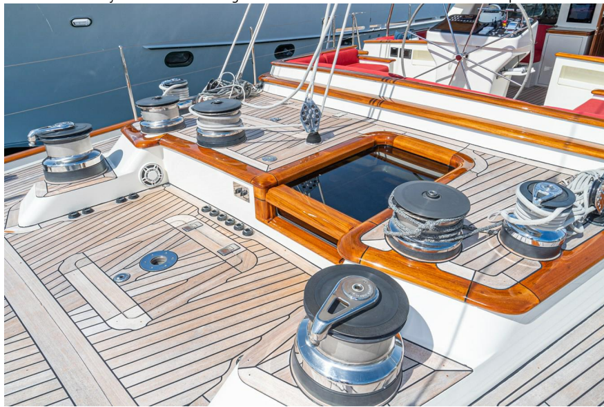
All Hydraulic Sailhandling Aft - Clear of Helm and Entertainment Cockpits
